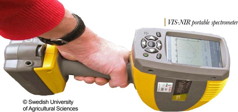
VIS-NIR portable spectrometer
